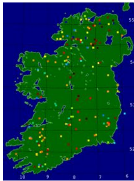
Fig. 2 Horizontal map of wind farm distribution according to their year of grid connection with colours following the colour scale, blue indicating connection before 1997, dark red in 2017-2018
